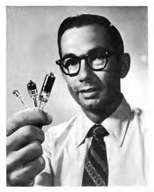
GORDON BOETTCHER (1312) displays a "family" of his Spryton devices. They perform switching functions in capacitor discharge circuits.
